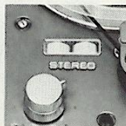
4. Electronic Beam Indicators ("magic eyes") with slow backward movement ensure correct recording level.
