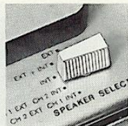
3. Loudspeaker selector with 5 positions controls both internal and external loudspeakers.
