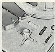
1. Central control lever (joystick) for sure, easy and quick tape transport. Eliminates the possibilities of error.
