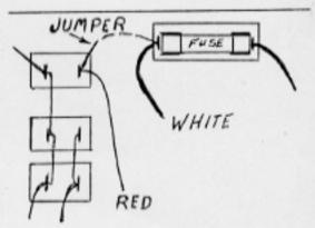
Install the jumper wire on all units received for service that have not been modified.
