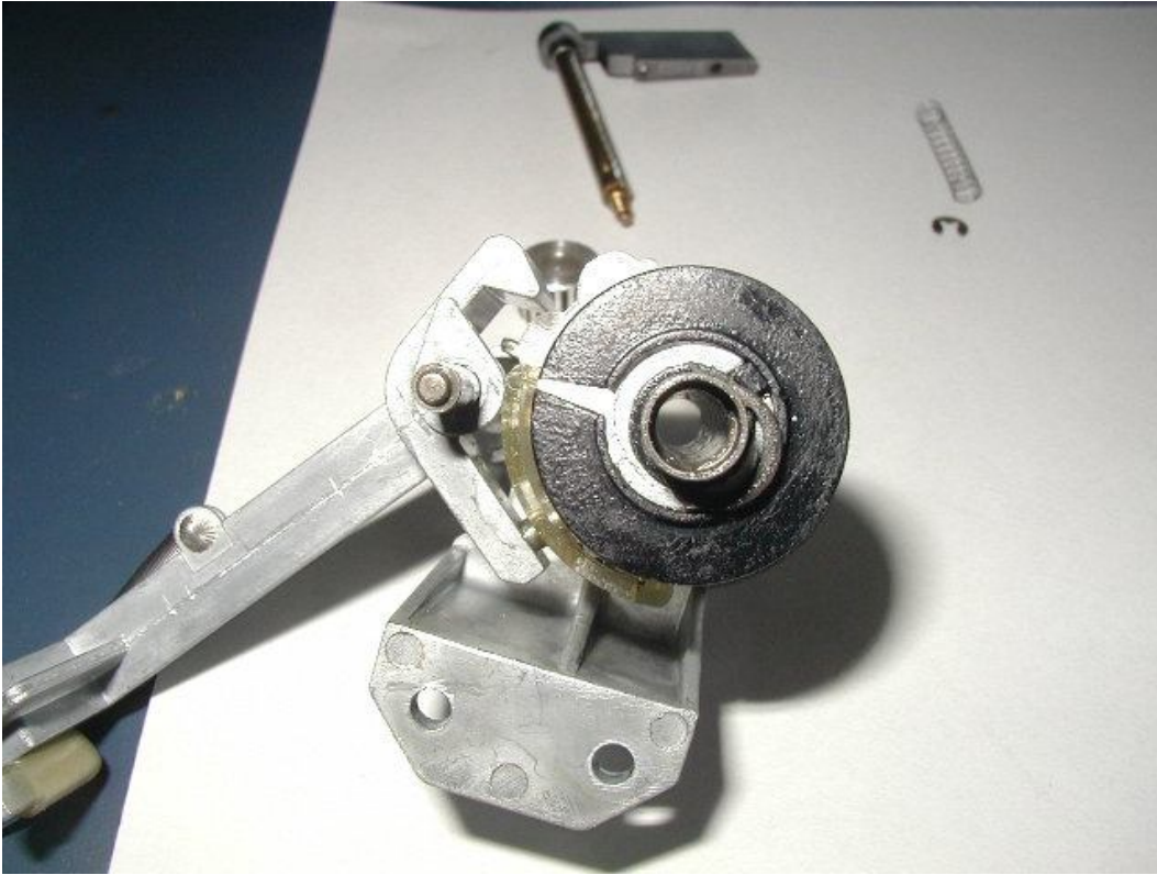
Large C-clip partially removed from pitch pointer...
