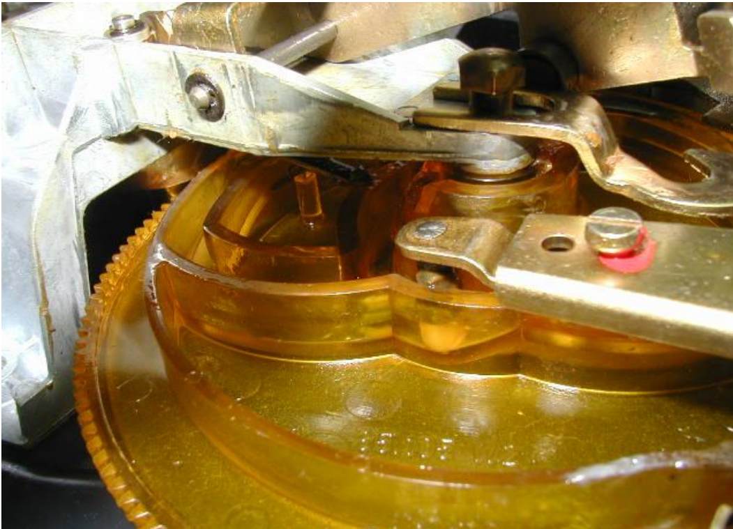
Lever pin in cam wheel track
