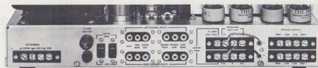
Rear panel of a typical Fisher stereo receiver, illustrating the simple, logical arrangement of all necessary connection points in a working stereo system.
