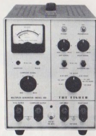
The Fisher Model 300 Multiplex Generator
