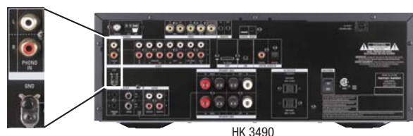
Figure 14 – Phono Inputs and Ground
