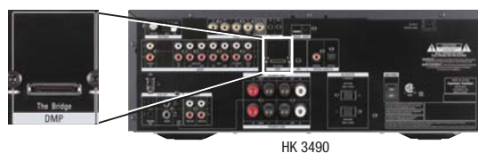
Figure 20 – The Bridge II Connection
