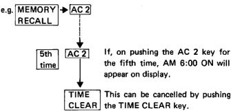
If, on pushing the AC 2 key for the fifth time, AM 6:00 ON will appear on display.
