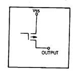
The O outputs have nominally 6002 on-state impedance
