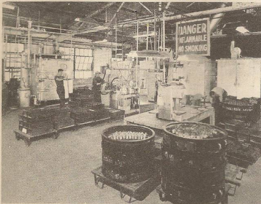
Vacuum tanks and ovens in a section of the impregnating facilities.
