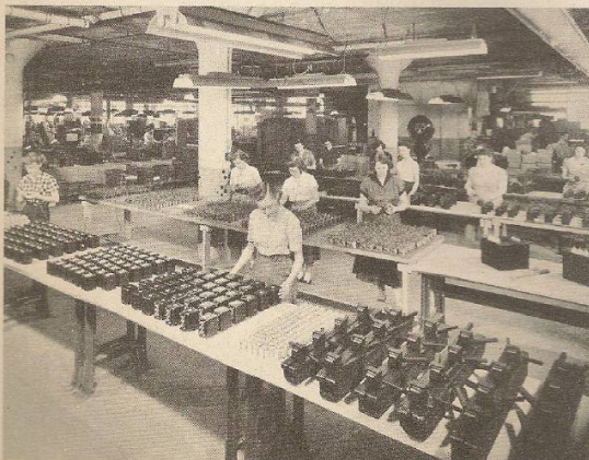
Final inspection where experienced inspectors check labels, leads, bushings, dimensional tolerances and finish.
